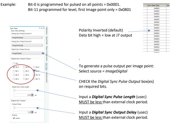
Condition: Ext-clock rate 200KHz, RF output channel delay = 0nsec. Programmed with SDIO bit 11 = level, SDIO Output Delay = 0.75usec (not 1.3 as shown above)
