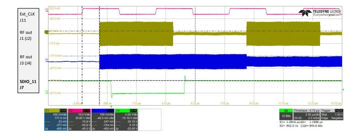
Condition: Ext-clock rate 200KHz, RF output channel delay = 0nsec. Programmed with SDIO bit 0 = pulsed, SDIO pulse width 0.5usec, SDIO delay = 0.75usec
