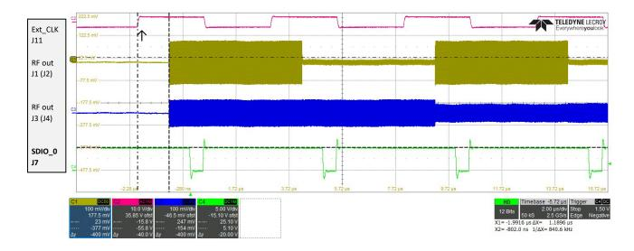
Note: the fixed 1.2usec latency from rising clock edge  $\uparrow$  to the active RF output, (no programmed Channel or RF delay)
